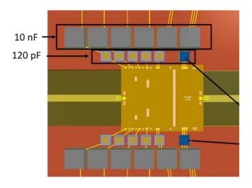
4 levels of decoupling capacitor have been used, 2 on the tab and 2 on the board. The first level is composed of 120 pF chip capacitors, the second level is composed of 10nF chip capacitors, the third level is composed of 100nF SMD 1210 capacitors and the fourth stage is composed of 1µF SMD 1206 capacitors. The first two levels should be as close as possible to the die. A 1K $\Omega$  resistor was added in series on each gate supply.
