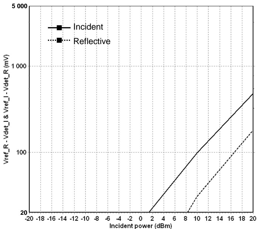
Incident and reflective power detection versus incident power @ 12GHz (Vdetect_I & Vdetect_R)
